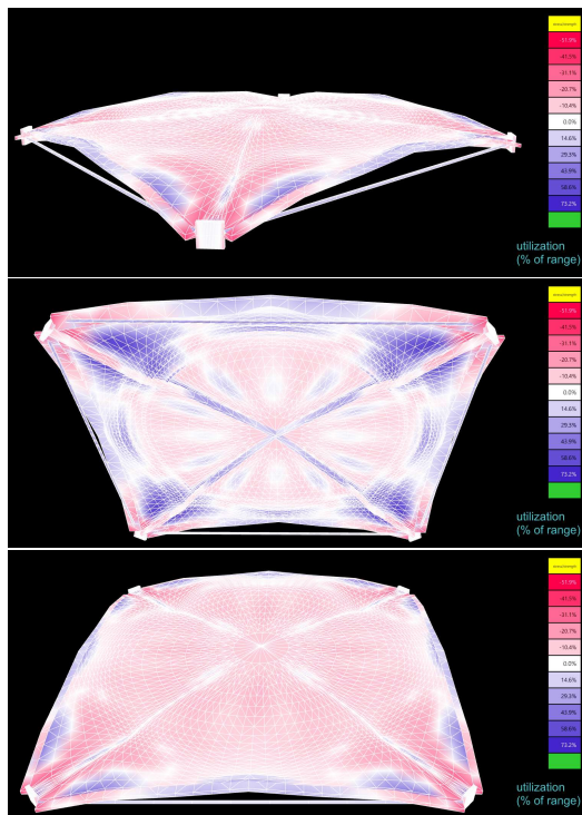
Figure 7: Utilization of slab under uniform load
