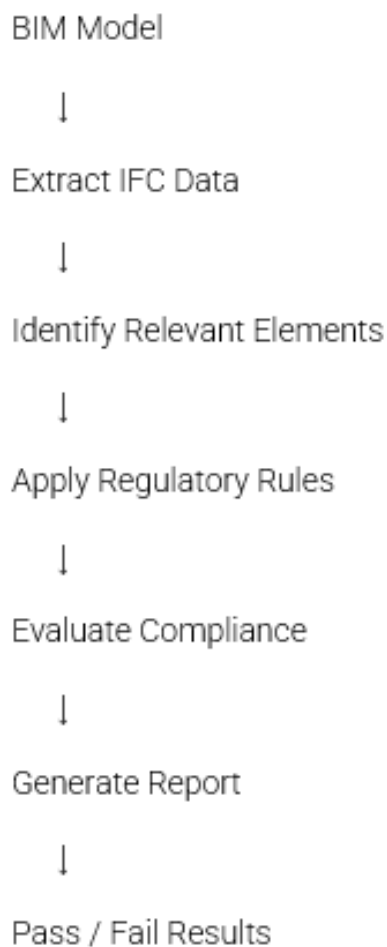
Figure 2. Simplified workflow of rule-based BIM compliance checking.
